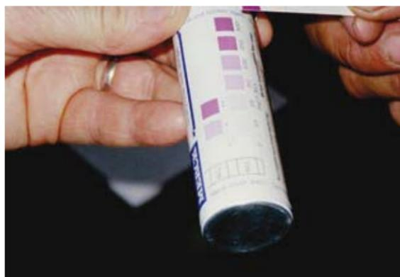
Example of a nitrate quick-test: this particular test showed that drinking water well had a very high level of nitrate
